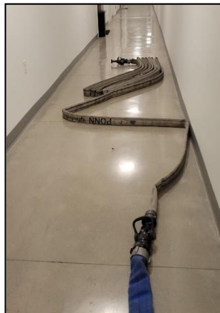
Photos 6-5, 6-6: 1-3/4" Corona bundle connected to the high rise-shutoff
