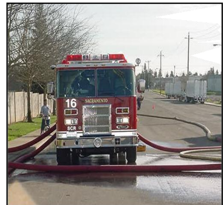
Photo 5-16: Multiple supply lines from different hydrants sharing the same water main.
