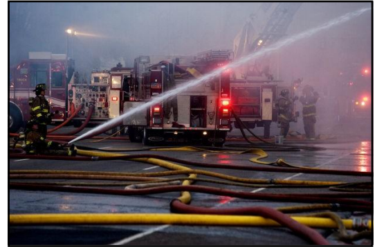
PHOTO 7-1: Heavy or advanced fire may require the use of master streams.
