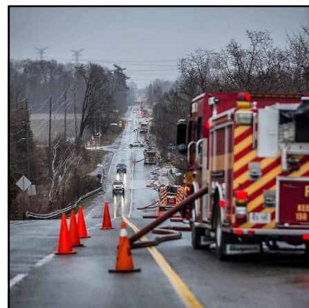
Photo 5-18: Relay pumping over long distances requires coordination.
