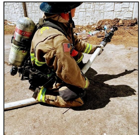
Photo 4-17: D' Clamp allows the nozzle reaction to be absorbed by the ground.
