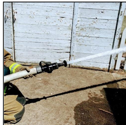
Photo 3-5: The solid stream from a smooth bore tip.
