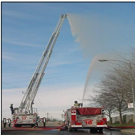
Photo 5-17: Multiple supply lines from different hydrants not sharing the same water main.
