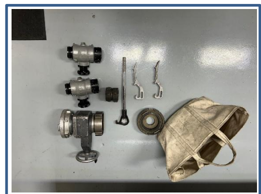
Photo 5-6: A typical hydrant bucket and its contents.
